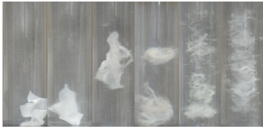
Figure 1. Break-up of nonwoven and dispersion of fibres in water at different stages
