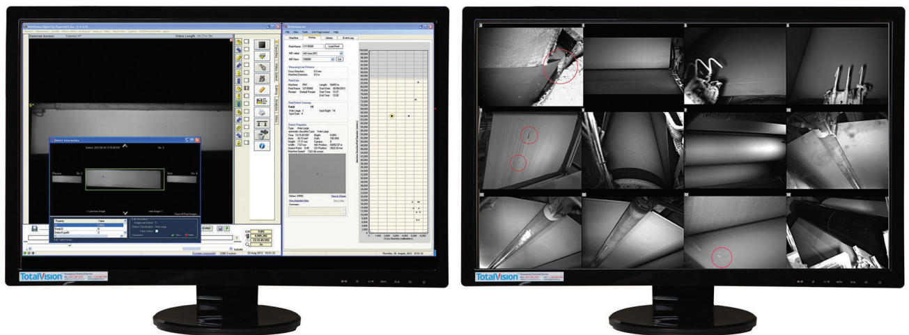
Figure 5. Example of a combined WIS (left) and WMS (right) operator control station display set-up providing total visibility to all of the machine cameras synchronised to the same piece of paper. Full two-way software integration provides automatic image transfer via pop-ups, as well as defect classification information, and other important variables to help speed up solving the root cause.
