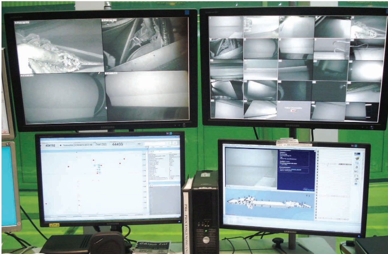
Figure 4. Shows how a fully integrated, single platform, web monitoring (WMS) and web inspection (WIS) operator station that allows a defect to be automatically transferred from the WIS to the WMS system synchronised to the same piece of paper. This allows for a rapid and accurate means for the user to find the source of the defect and to eliminate it. A single keyboard and mouse is able to operate both systems.
