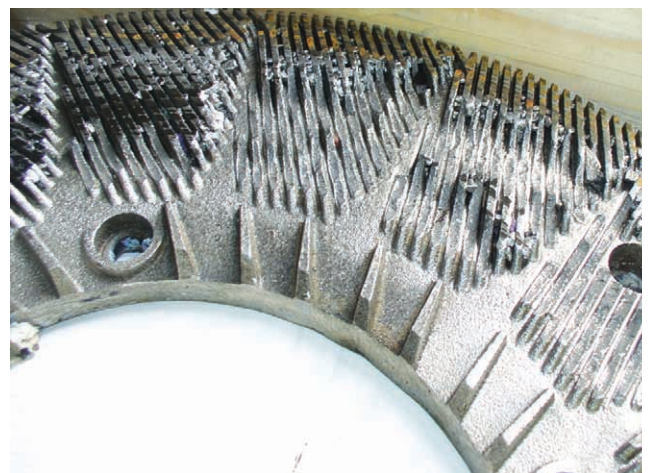
Figure 3. Damage from a large contaminant entering the refiner
