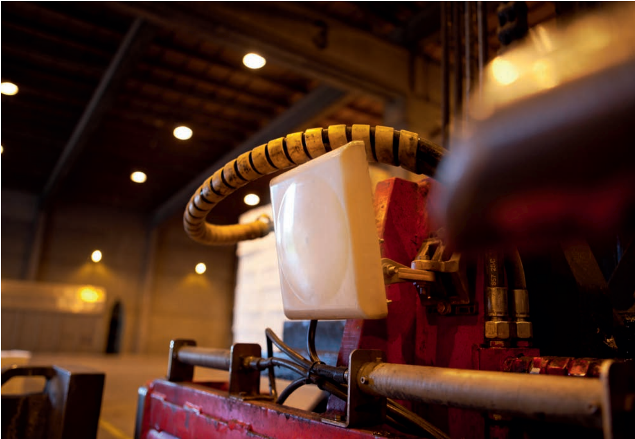
Bottom left: Collecting electronic tracking information with a forklift reader Left: A forklift reader at the Metsä Fibre Rauma mill's warehouse Below: A portable RFID reader
