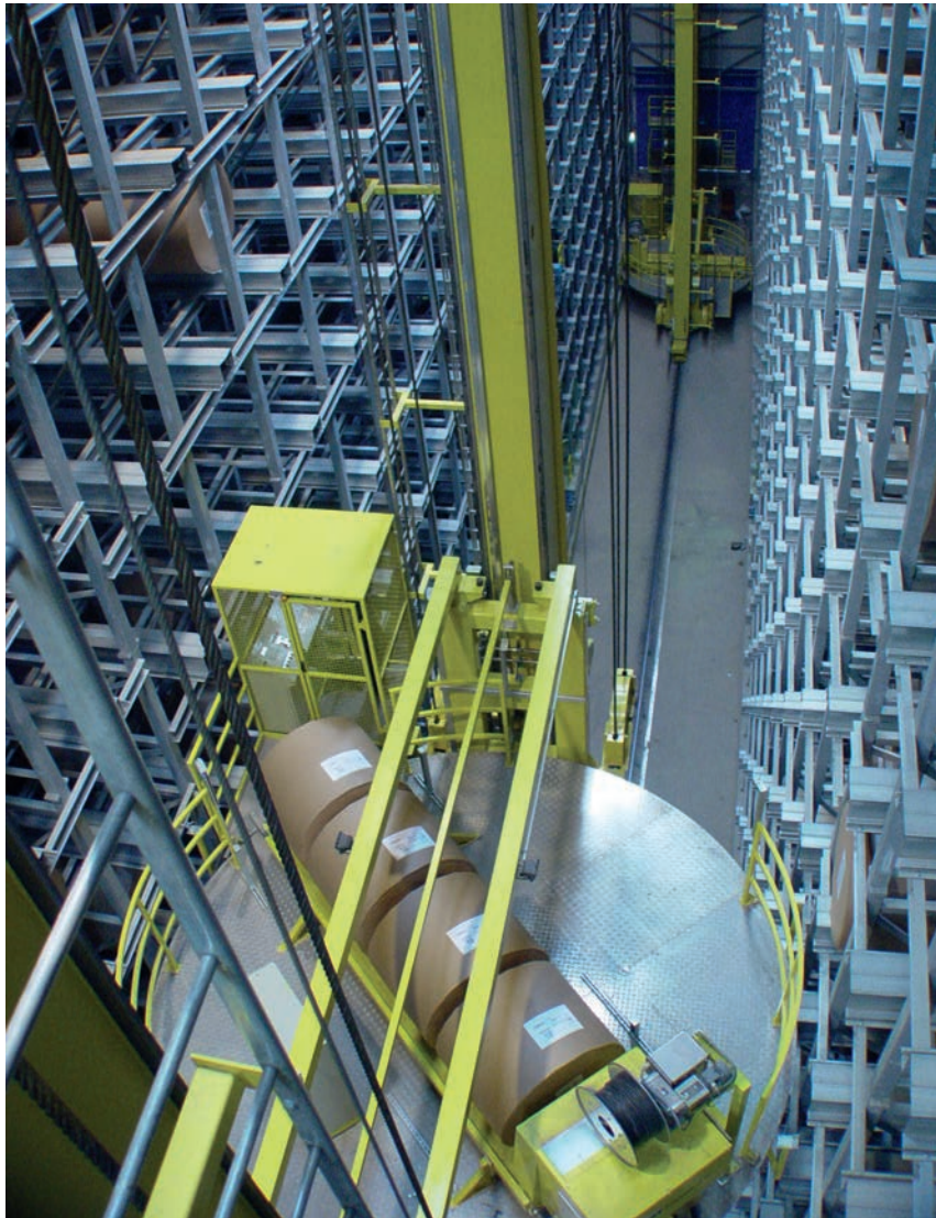
Figure 4 Multi-roll handling is the key for high handling capacity. This combined to the hig-bay storage's sorting capacities means practically limitless automatically controlled material stream.
