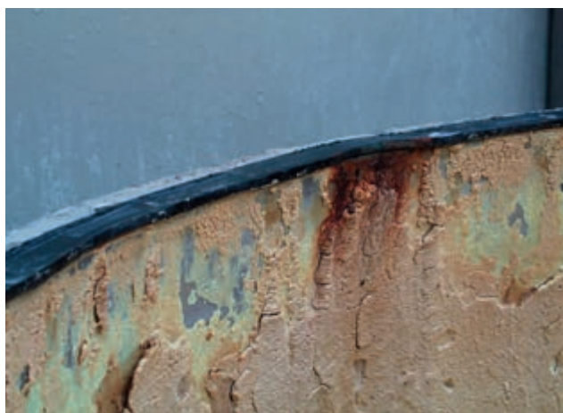
Figure 4 : Examples of Possible Microbiological Contaminations in Standard Starch Systems
