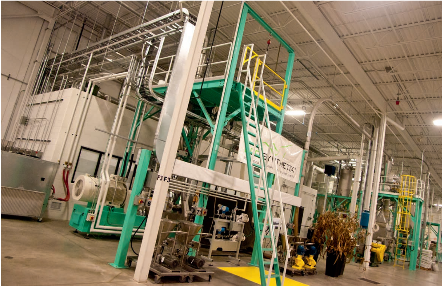
Figure 1 ECOSYNTHETIX pilot reactive extrusion line in Burlington, Ontario supports the company's new product development efforts
