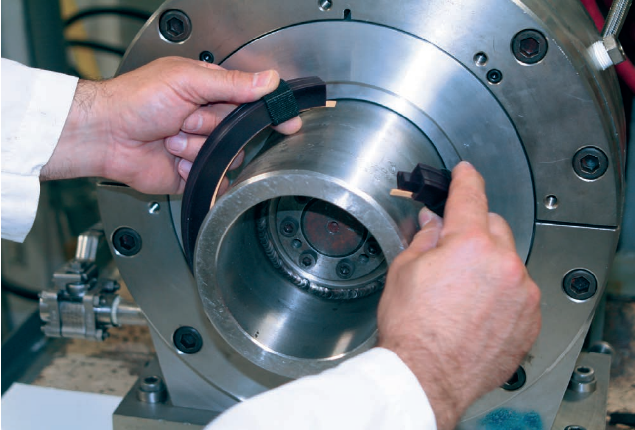
Figure 8 Chesterton 33K Split Bearing Protector
