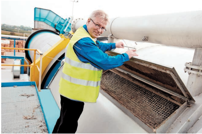
“The new generation design is better at deflaking and defiberising hard-to-pulp wastepaper furnishes.” Kimmo Vanhala, FibreFlow Drum Product Manager at ANDRITZ, inspects the screening zone of the Drum.
