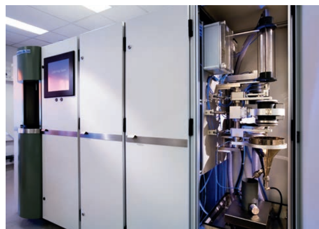
Picture 3 A paper sample is fed into the system and measurements start automatically
