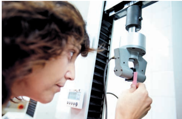
Pilar Carnicé performs a paper tensile strength test.
