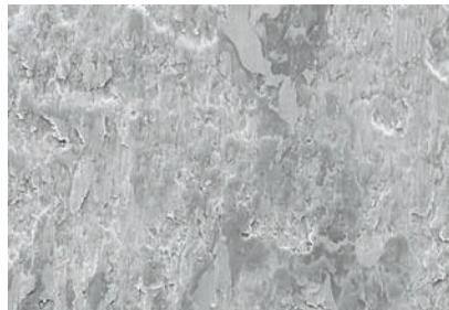
Microwelding on steel blade due to adhesive wear
